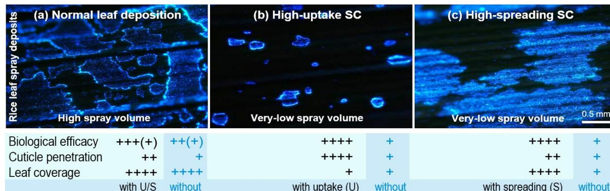
Foliar spray deposits on rice plants illustrating different deposit structures (coffee rings/uniform) and distributions for high (a) and low spray volumes with uptake promoting (b) and high spreading surfactants (c).
